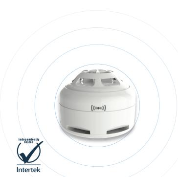
Each detector features a multi colour LED for status indication and dual fire LEDs for fire indication when in pre-alarm or alarm mode. The wireless addressable base enables communication between the detector and the control panel – this is achieved through the Cygnus wireless protocol. This device is battery-powered and has a minimum three year battery life.
