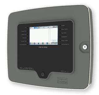
What's more, it is designed and manufactured to meet EN 54-2, EN 54-4 and EN 54-25 standards. It can also be installed, serviced and maintained in accordance with BS 5839-1. The control panel transmits wirelessly and is mains powered with a battery backup facility, built to last up to four days. Control Panel messages include alarms, pre-alarms, low battery alerts, and faults – all identifiable by location.
